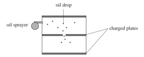
The radius of an oil drop had to be determined so that its weight could be calculated.
