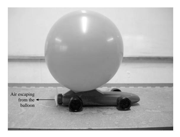
When the air in the inflated balloon is released, the car starts to move forwards.
